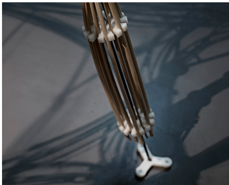
Figure 4.3a: Steel rod and ball joint detail activated by “thigmotropism” in the generative algorithm, used in climbing and secondary environmentally responsive connections. Photo by Anders Ingvartsen
