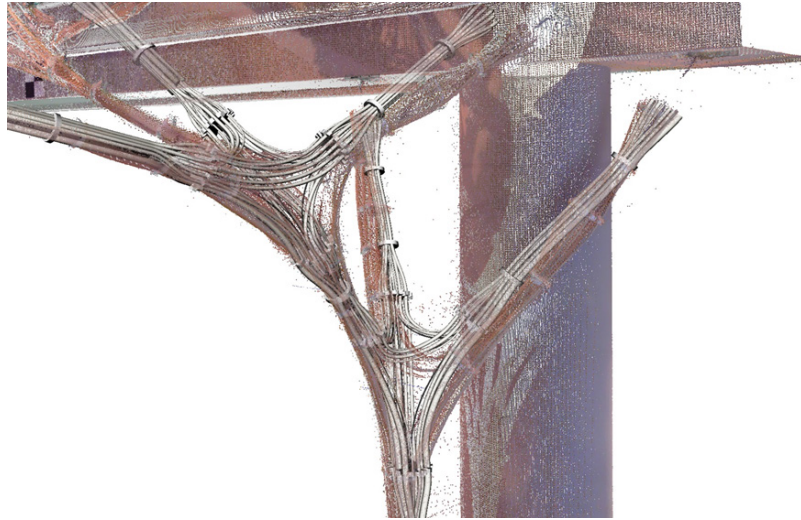
Figure 4.15: Comparison of digital model to 3D scan of final installation. (Martin Tamke)
