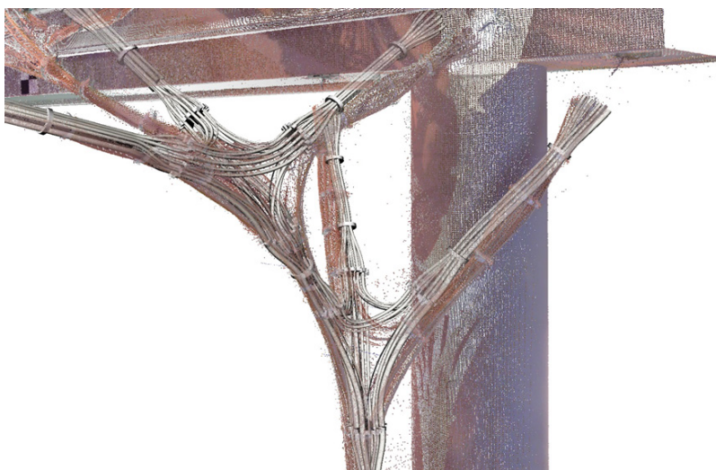
Figure 12: Generated detailed model overlaid with 3D scan of built installation (Martin Tamke)
